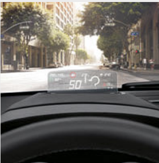
○ The Head-Up Screen puts vehicle information and, in combination with a smartphone interface, navigation information into the driver's line of sight.
