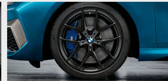
○ Sporty 18" M Performance forged wheels V-spoke style 554 M in Jet Black matt. TPMS summer complete wheel set, wheel size 8J x 18.
