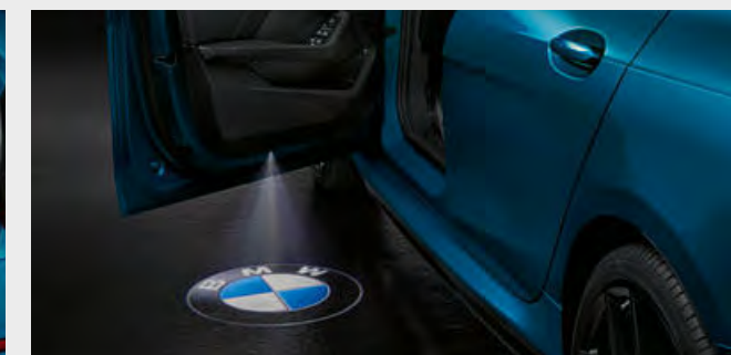
○ The LED door projectors are activated when the doors are opened. They project an image onto the ground next to the car using an interchangeable slide.
