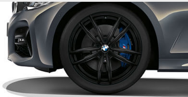
□ 19" M light alloy wheels Double-spoke style 791 M Jet Black uni with mixed tyres and runflat tyres¹, burnished, front 8J x 19 with 225/40 R19 tyres, rear 8.5J x 19 with 255/35 R19 tyres.
