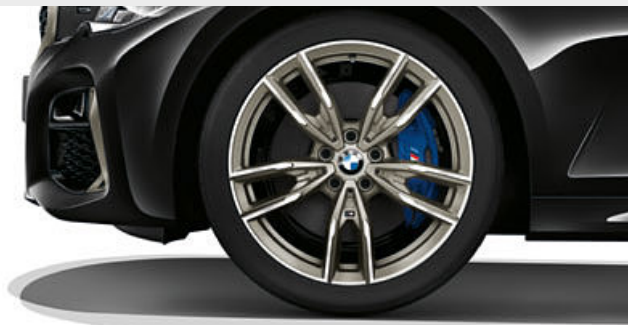
□ 19" M light alloy wheels Double-spoke style 792 M Bicolour Cerium Grey with mixed tyres and runflat tyres²*, burnished, front 8J x 19 with 225/40 R19 tyres, rear 8.5J x 19 with 255/35 R19 tyres.
