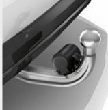
☐ The Trailer tow hitch with electrically adjustable tow ball and trailer stability control is approved for heavy loads of up to 2,400 kg.
