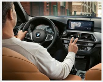
☐ With BMW Gesture Control\*, certain functions can be operated by means of defined hand movements. For certain operations the system will for example recognise gestures such as 'swiping' or 'pointing' for accepting or rejecting an incoming call, or circular motions of the index finger to adiust volume
