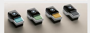
☐ The Ambient Air Package\* comprises a fragrance dispersal function and an air ionisation function. There are eight fragrances to choose from, all specially composed for the vehicle
