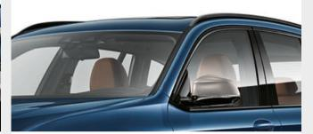
☐ The acoustic glazing on the front side windows complements the acoustic glazing on the front windscreen and significantly reduces the level of noise for everyone inside the vehicle. It minimises noise created by the outside surroundings and flow of air, as well as by the engine, tyres and windscreen wipers. Music listeners and hands-free device users in particular will appreciate the difference this makes.
