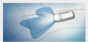
☐ The **LED headlights with cornering lights**<sup>2</sup> generate a bright and efficient bi-LED light for low and high-beam headlights. The bend lighting and cornering lights with LED technology allow for adaptive light distribution with increased side illumination for city driving. The LED daytime running lights and parking lights in the light tubes of the main headlights create a distinctive feature characteristic of a BMW.
