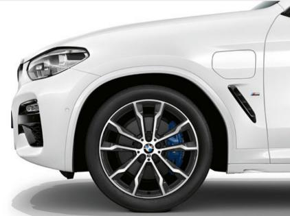
The port for external charging of the high-voltage battery is located behind a flap on the vehicle's front side panel on the left.
