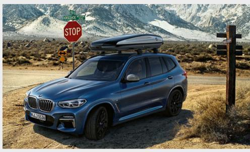
O This contemporary roof box in Black with titanium silver side trims has a 520-litre capacity and fits all BMW roof rack systems. It can be opened from both sides and features triple central locking on each side which makes it easy to load and provides anti-theft locking.
