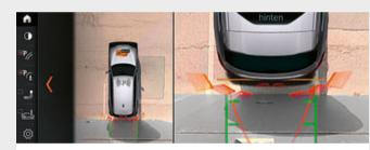
☐ The equipment package Parking Assistant Plus\* makes parking and manoeuvring the vehicle easier. It features Surround View including Top View, Remote 3D View, PDC as well as a lateral parking aid, the Active PDC emergency braking function and the Parking Assistant with linear guidance that provides fully automatic parking both parallel and perpendicular to the road.
