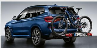
O The Pro 2.0 rear bicyle rack is lightweight yet sturdy and can carry up to 60kg. Exceptionally easy to use, it carries two bicycles or e-bikes (can be extended to accommodate three bicycles). Its tilt function also allows easy access to the luggage compartment at all times
